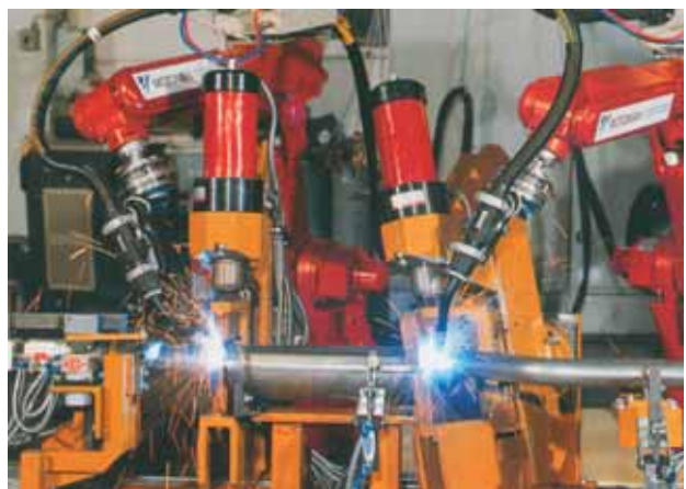
Welding fixture for exhaust components
