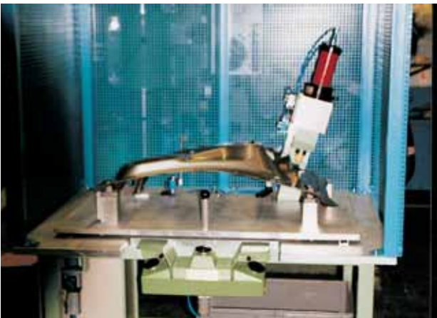
Device for holes Ø 8 in sheet metal
