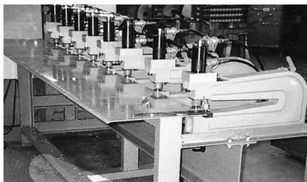
Hydraulic short-stroke cylinders for DE-STA-CO punching units in a series punching fixture
