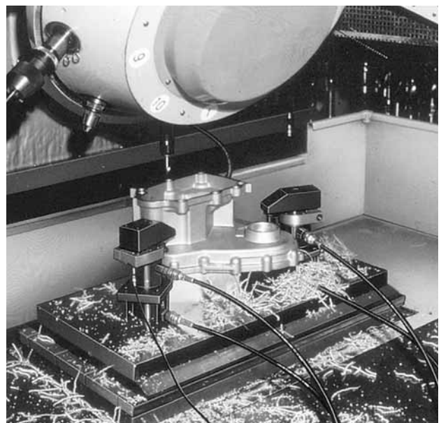
Hydraulic swivel clamp, double action (see catalogue pages 24.1 to 24.4) for clamping cast parts on a milling fixture
